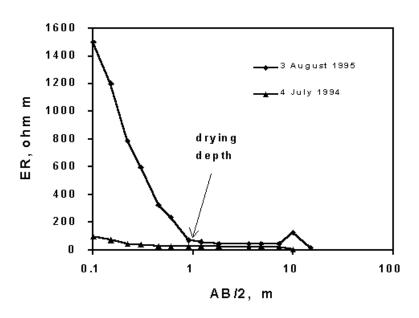
(Figure, VES for 4 July, 1994). In extremely dry years as in the summer of 1995 in Moscow area, Russia, the upper 50-cm layer of peat soil dried almost to the wilting point, causing an increase of electrical resistivity up to 1,500 ohm m. The drying depth was precisely determined with the VES interpretation. The estimation of drying depth with computer interpretation of VES was verified with direct water content measurements in soil samples collected from the different soil layers.
